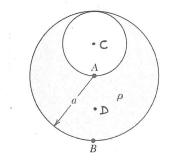
(a) A solid non-conducting sphere of radius a is filled with positive charge of uniform charge density  $\rho$ . Then a smaller sphere of radius  $\frac{a}{2}$  is carved out as shown in the figure and left empty. What are the direction and magnitude of the electric field **E** at *A*? At *B*?
